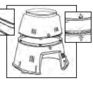
Step 3 - Check the outside and insidewith your hand to ensure the 6 tabs line up with the 6 slots.
