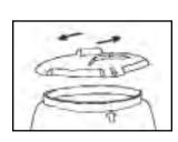
Step 2 – Place the bottom section on the ground, and set the top section on top of it. IMPORTANT: Make sure that the arrows on the the top and bottom sections line up. Also, the bottom of the top section should sit in the groove on the top of the bottom section.
