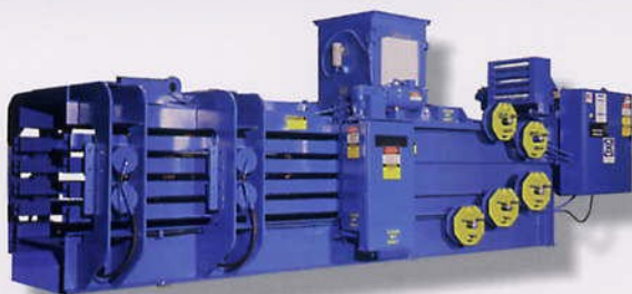
Corrugated / Folding Carton Plant Baler - 1500 lb. bales
